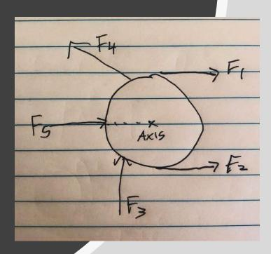
1. Tell whether each force in the diagram creates a positive torque, negative torque, or zero torque about the axis.
